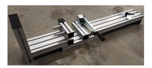
This accessory is designed in order to cut doctor blades with different sizes in a short time.
